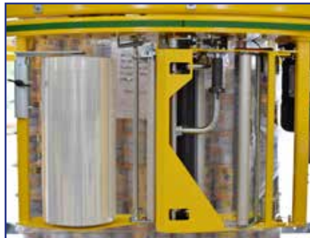
1. The patented Easy S film carriage with easy-load feature ensures quick change over and reduces downtime. The carriage also features a very efficient power pre-stretch film system.
